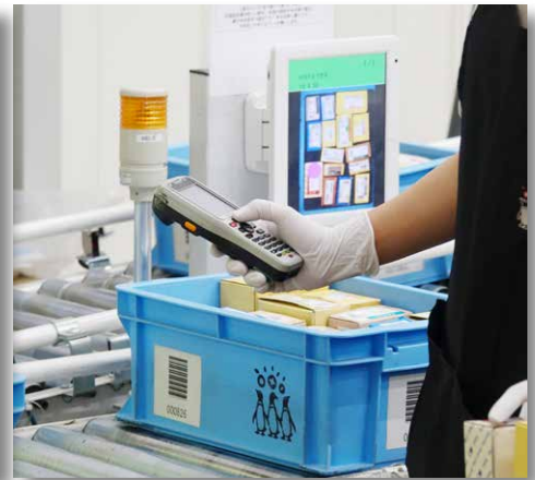
Fig. 18. The monitor displays a red dot on a questionable package in the bucket after a barcode scan
