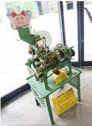
Fig. 5. Wood screw threading machine from the 60s displayed at the entrance
