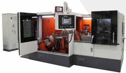
1D2B COMBINED HEADER - KSP12
